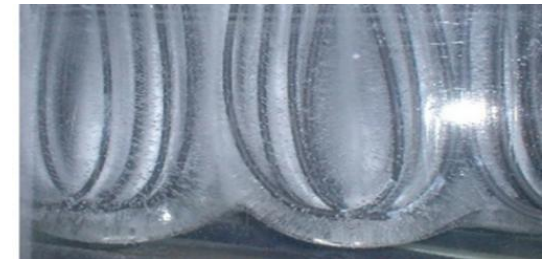
Layer of ice forming around the heat exchanger tubes.
